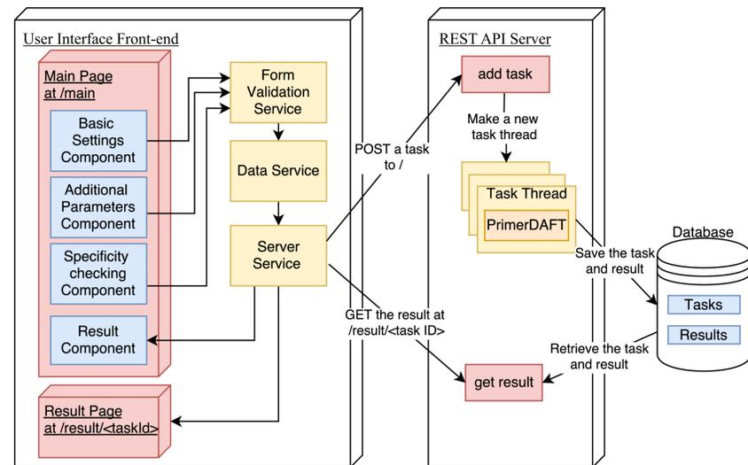
Figure 6: Block Diagram showing how the tool works
